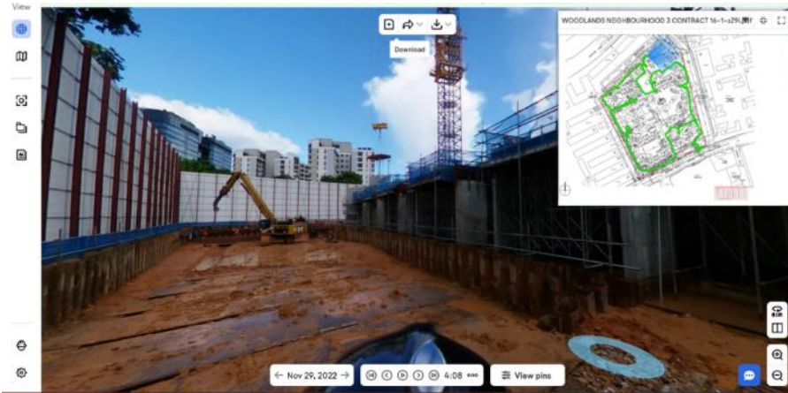
1. Using 360 Capture to check completeness of site before inspection
