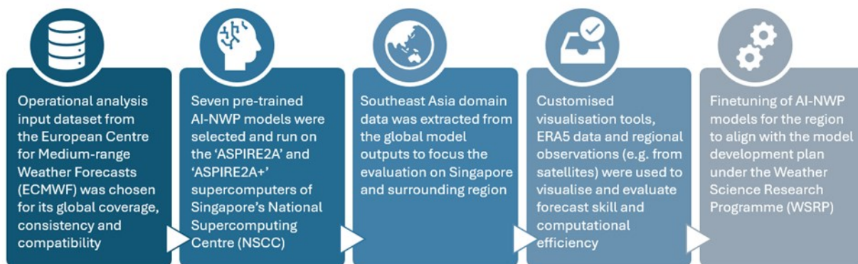
Figure 3. The benchmarking workflow was structured to evaluate the forecast skill and computational efficiency of selected pre-trained AI-NWP models, using a combination of global reanalysis data, regional observations, and visualisation tools tailored for evaluation.
