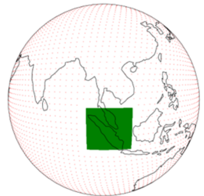
Figure 7. A stretched grid showing the boundary between global and regional domains.
