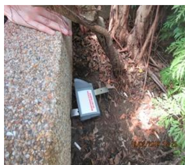
Sensor placed on the ground near potential rat runways and with lesser human traffic.
