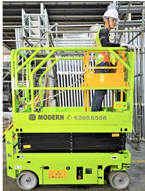
Example of approved access deck
