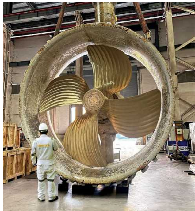
Home-grown firm Mencast Marine partnered with A*STAR and the National Additive Manufacturing Innovation Cluster (NAMIC) to produce Singapore's first additively manufactured marine propeller in 2023.
