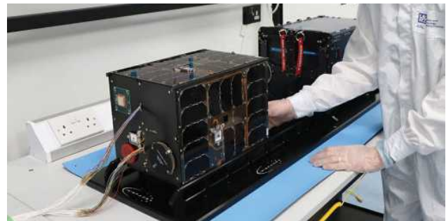
SpeQtre was developed by SpeQtral, a company spun off from CQT, in collaboration with the UK Science and Technology Facilities Council's (STFC) RAL Space. The SpeQtre satellite carries advanced quantum hardware designed by SpeQtral to explore secure space-based quantum communications. It aims to demonstrate the exchange of quantum information from a CubeSat roughly the size of a microwave oven.
