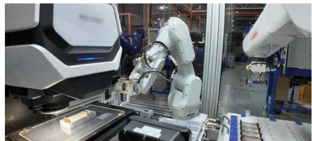
Nozzle Guide Vane (NGV) and Stator Dimensional inspection system developed through the Smart Manufacturing Joint Lab, deployed at SAESL's MRO facility. Photo credit: A*STAR
