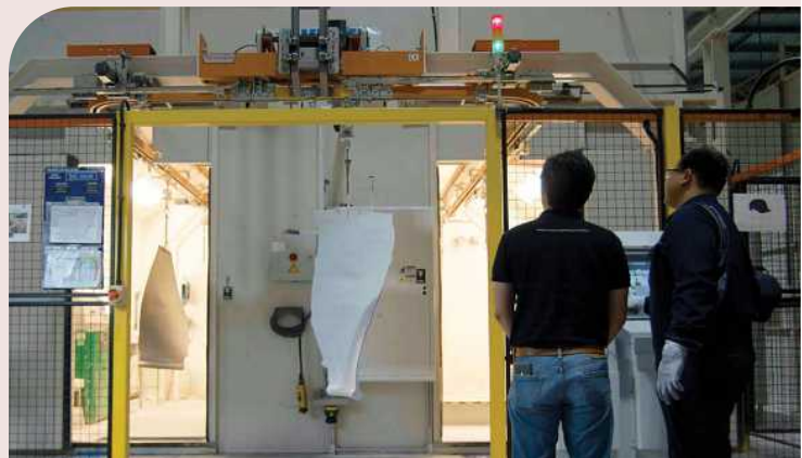
Automated boron nitride spray system developed through the Smart Manufacturing Joint Lab for Rolls-Royce's Seletar facility.
