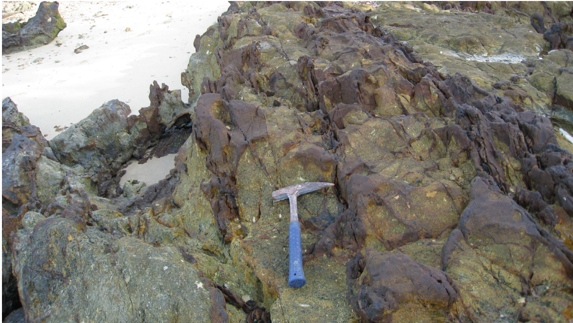
Figure 14. Near vertical-dipping coarse cross bedded sandstone outcrop. Photo credit: Dr Stephen Chua, EOS, NTU.
