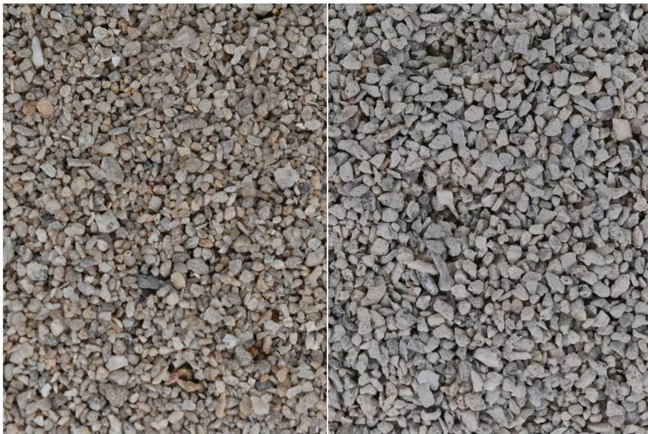
Natural sand (left) and alternative sand created by combining captured carbon dioxide with incineration bottom ash. PHOTOS: A*STAR
